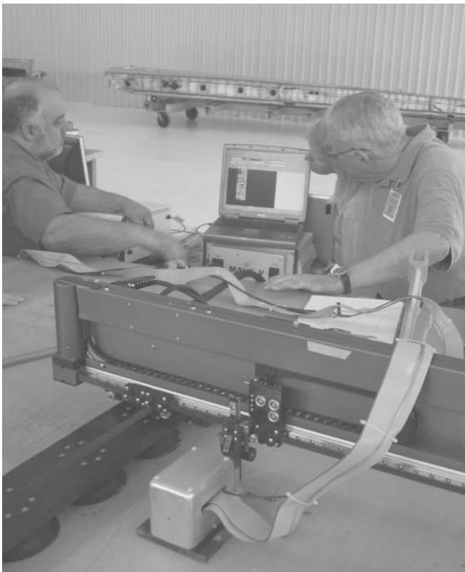
Figure 4.52. Prototype MR Sensor Array Contained in a Head Being Translated Over a Specimen by a MAUS Platform to Produce Real-Time Images.
