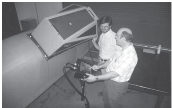
Figure 4.36. D-Site™ System Positioned on an EC-135 Aircraft Radome for Inspection.
