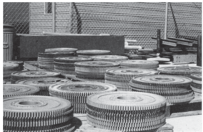
Figure 4.14. Turbine Engine Disks “Retired” from Service after Reaching an Analytically Prescribed Conservative Usage Life.
