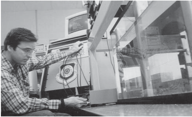
Figure 4.42. Fine-Tuning a Material Characterization Test in the High Precision Scanning Acoustic Microscope.
