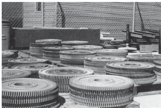
Figure 3.9. Turbine Engine Disks “Retired” from Service after Reaching an Analytically Prescribed Conservative Usage Life.
