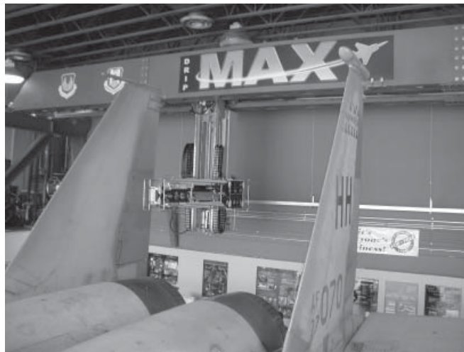
Figure 4.38. Automated High Resolution Real-time Multi-Axis Radiography (MAX) System for On-Aircraft Nondestructive Inspection. The System is Shown Scanning an F-15 Vertical Tail.
