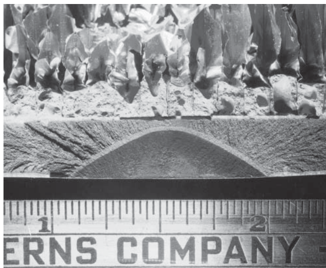
Figure 3.3b. Undiscovered Elusive Manufacturing-Induced Flaw (Dark Half Ellipse) Extended by Fatigue Growth (Narrow Lighter Band) Causing Failure.
