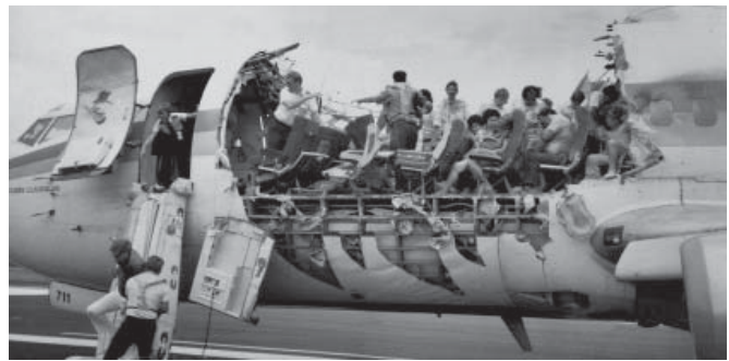
Figure 3.10. Near Catastrophic Failure of Upper Fuselage Structure of Aloha Airlines Boeing 737 in 1988.
