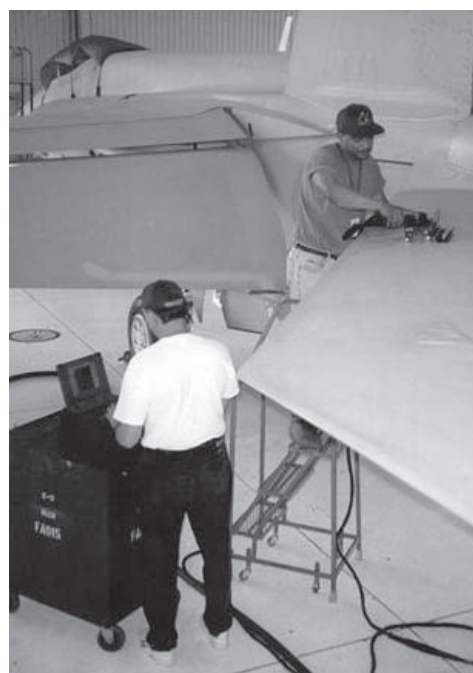
Figure 4.33. Mobile Automated System (MAUS) IV Scanning On-Aircraft Airframe Component.
