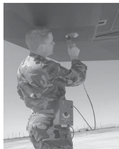
Figure 4.41. Evaluation of LO Component on F-117 Stealth Aircraft with a Point Inspection Tool Developed Under Contract by Lockheed Martin Skunk Works.
